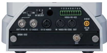
BRC-300 rear panel with the optional BRBK-302
